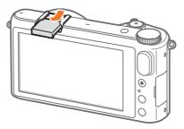
Mount the GPS module by sliding it into the hot-shoe.
