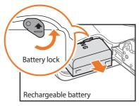
Slide the lock up to release the battery.
