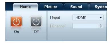
You can power on or off a selected device or change the input source or volume of the device. Choose display devices from the list of sets, and select the **Home** tab.
