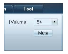
The volume can be changed or the sound can be muted only for displays that are turned on.
