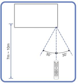
Use the remote control within 7m to 10m from the sensor on the product at an angle of 30° from the left and right.
