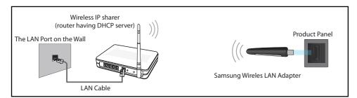
Samsung's Wireless LAN adapter is sold separately and is offered by selected retailers, Ecommerce sites, and Samsungparts.com. Samsung's Wireless LAN adapter supports the IEEE 802.11a/b/g and n communication protocols. Samsung recommends using IEEE 802.11n. When you play video over a network connection, the video may not play smoothly.
