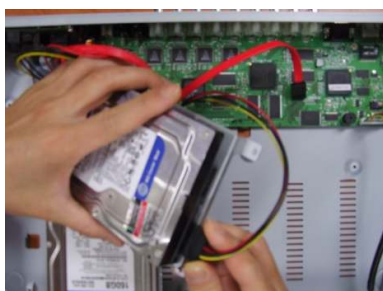
[Connecting power cable]
