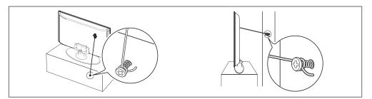
**4.** Verify all connections are properly secured. Periodically check the connections for any sign of fatigue or failure. If you have any doubt about the security of your connections, contact a professional installer.
