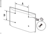
Remove the screws in the mounting holes before you install the wall mount.
