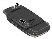
2. Lift the battery from the bottom end (see arrow 1) and remove.
