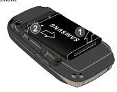
3. Slide the battery cover up until it snaps into place.
