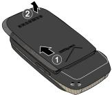
Insert the top end of the battery into the phone housing using the directional arrow printed on the battery. The gold contacts at the battery end must align with contacts on the phone. Push bottom end of the battery down until it snaps into place.
