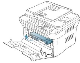
Thoroughly roll the cartridge five or six times to distribute the toner evenly inside the cartridge.
