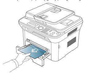
If the paper does not move when you pull, or if you do not see the paper in this area, check the fuser area around the toner cartridge (See "Inside the machine" on page 93).
