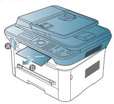
After getting a printout, close the scan unit by pressing the scan unit close button.
