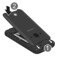
2. Press along the edge of the back cover (3) until you have a secure seal.
