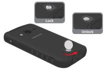
**2.** Remove the back cover by inserting a fingernail into the slot on the top of your phone (1).
