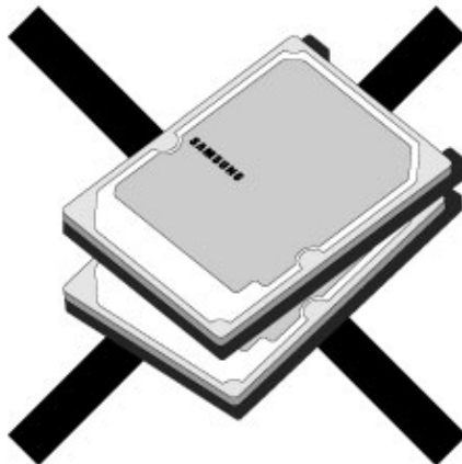
Fig. 9-3: HDD handling guide -Do Not Stack!
