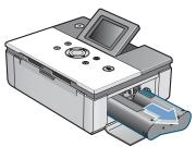
4 After removing the cartridge from its package, rotate the roller to smooth out wrinkles or uneven areas in the film. If the film is not even, it could be damaged during installation.
