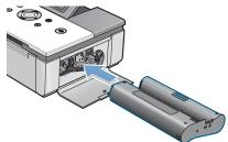
4 Make sure that the cartridge is under the lever and then close the side cover.
