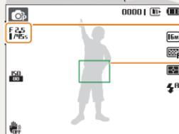
The camera sets the aperture value and shutter speed automatically.
