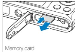
Push the card gently until it disengages from the camera, and then pull it out of the slot.
