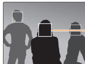
The face nearest the camera or nearest the center of the scene appears in a white focus frame and the rest of the faces appear in gray focus frames.
