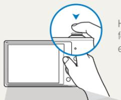
Half-press [Shutter] and adjust the focus. The camera adjusts the focus and exposure automatically.
