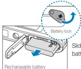
Slide the lock up to release the battery.
