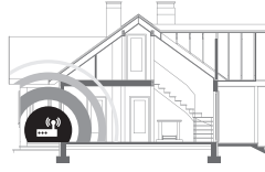
Unsuitable router position
