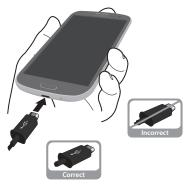
Note: This illustration displays both the correct and incorrect orientation for connecting the charger. If the charger is incorrectly connected, damage to the accessory port will occur therefore voiding the phone's warranty.
