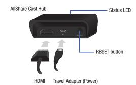
Connect the AllShare Cast hub to a power source via the USB Travel Adapter.
