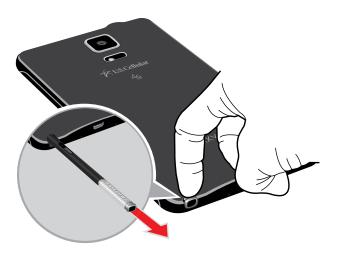
**Caution**: When you insert the S Pen into the slot, insert the S Pen's tip first. Failure to do so can cause the S Pen to become stuck. Forcefully detaching the S Pen from the slot may cause damage to the S Pen and your device.
