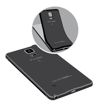
2. Press along the edge of the back cover until you have a secure seal.
