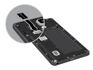
**Caution**: If the memory card is not inserted correctly, the device cannot detect it. Reorient the memory card and place it back into the slot if it is not detected.
