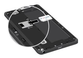
**Caution**: If the SIM card is not inserted correctly, the device cannot detect it. Reorient the SIM card and place it back into the slot if it is not detected.
