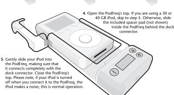
**6.** Hook the top of the latch over the hook on the top part of the PodFreq.
