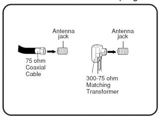
Connect the 75 ohm cable from the combination VHF/UHF antenna to the antenna tack.
