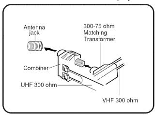
Connect the UHF 300 ohm twin-lead wire to the Combiner (not supplied). Connect the VHF 300 ohm twin-lead wire to the 300-75 ohm Matching Transformer. Attach the Transformer to the Combiner, then attach the Combiner to the Antenna Jack.
