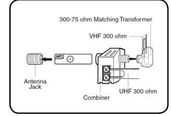
Connect the UHF 300 ohm twin-lead wire to the Combiner (not supplied). Connect the VHF 300 ohm twin-lead wire to the 300-75 ohm Matching Transformer. Attach the Transformer to the Combiner, then attach the Combiner to the Antenna Jack.
