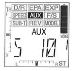
2) Press the +/INC or DEC/- keys to choose the Step value you would like to program. The higher the number, the more the Auxiliary Channel 3 servo travels with each press of the +/INC or DEC/- keys and the lower the number the less the Auxiliary Channel 3 servo travels with each press of the +/INC or DEC/- keys.
