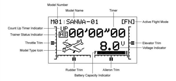
Active Flight Mode: Displays the Flight Mode number that is currently Active.
