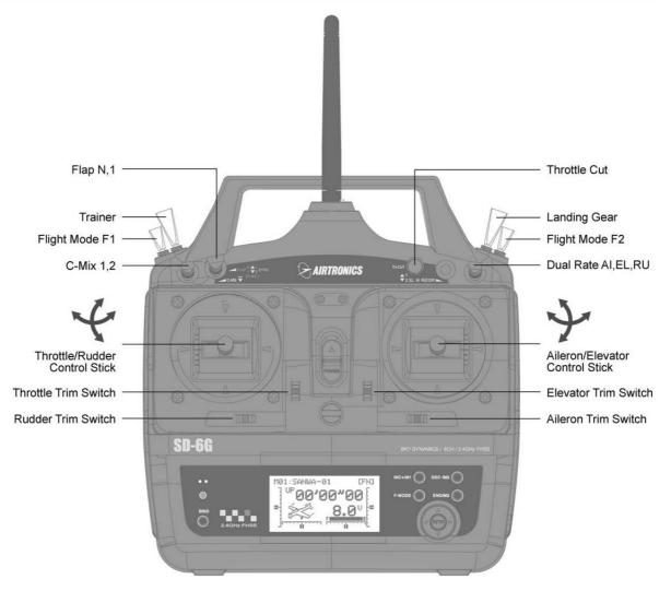
When any switch is moved into the Up or Forward position (pushed away from you), this is considered the OFF position. When moved into the Down position or Back position (pulled toward you), this is considered the ON position.
