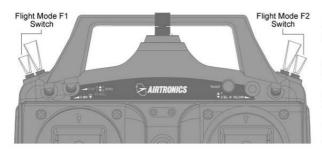
Flight Modes are turned ON and OFF using the two Flight Mode switches, as described below:
