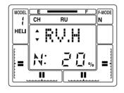
Use the INC +/YES or DEC -/NO key to change the default value if you desire to do so for any of the three flight modes. In this example, we have set RV.H for the Normal flight mode to + 25%.
