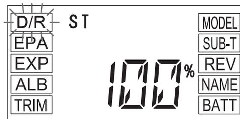
2) Press the INCREASE or DECREASE keys to change the Steering Dual Rate percentage value. When the Steering Dual Rate percentage value is decreased, steering servo travel is decreased. When the Steering Dual Rate percentage value is increased, steering servo travel is increased.
