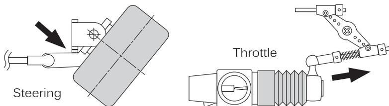
**!** If you're using an electronic speed control, the Throttle Forward and the Throttle Brake End Point Adjustment percentage values are both generally set to 100%, although the Throttle Forward direction may need to be increased to achieve full power. In some cases the End Point Adjustments can also be set directly via the electronic speed control.
