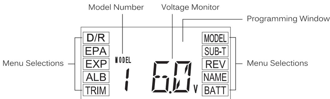
**Model Number:** Displays the model that is currently loaded into memory. Up to 10 different models can be stored.
