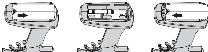
2) Install four fresh 'AA' Alkaline batteries into the battery holder, making sure that the polarity is correct. The direction that each battery should be installed is molded into the bottom of the battery holder (+ positive and - negative).
