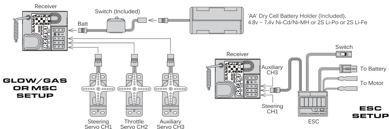
**!** Do not use servos rated for 4.8 or 6.0 volts with a 2S Li-Po or Li-Fe receiver battery pack or damage to the servos could result.
