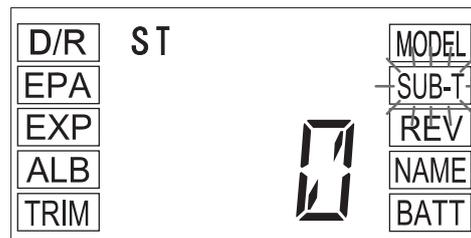
2) Press the INCREASE or DECREASE keys to adjust the Steering Servo Sub-Trim value either Right or Left to center the servo horn (or servo saver). The direction will differ based on the steering channel's Servo Reversing setting.
