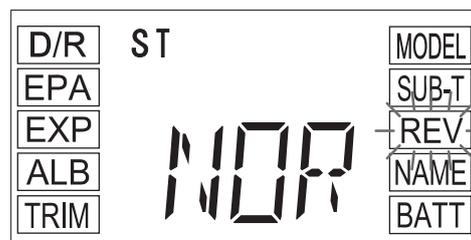
2) Press the MENU UP or MENU DOWN keys to choose which channel you would like to change the Servo Reversing value for, then press the INCREASE or DECREASE keys to change the direction of servo travel.
