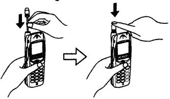
Move it straight down by pulling on a lower part of the antenna.
