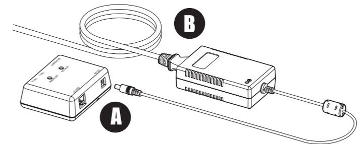
The SOMApport takes up to five minutes to start, connect to your service provider's network, and acquire a radio signal. The light on the power supply indicates whether or not it is receiving power. Wait until the Network light on the top of the SOMApport turns green before you begin connecting equipment to the SOMApport.
