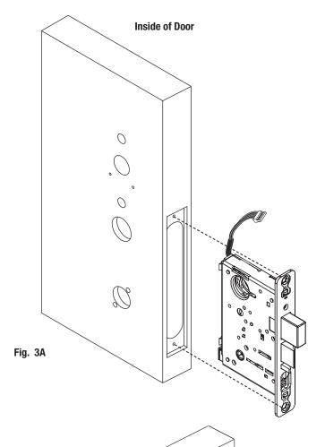
2. Hold lock body loosely in place with (2) lock body screws.
