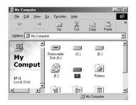
■ Caution: The new hard disk which doesn't have FDISK and FORMAT, can not be recognized in "my computer" If you want to FDISK and FORMAT, you have to follow the way in "NO. 6 the way of PARTITION and FORMAT" Then the drive will be installed in "my computer"
