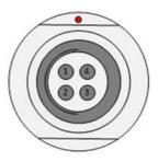
Note<sup>\*\*</sup>) Both PWR pins 1&2 must be connected! Note<sup>\*\*\*</sup>) Both GND and pins 3&4 must be connected!
