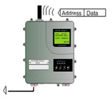
Reception addressing has been set ON, but both the primary and secondary RX addresses of the radio modem are different from the address of the received data packet.
