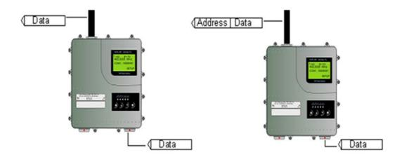
Transmission address has been set OFF. Radio modem will transmit the data packet as such. Transmission addressing has been set ON. The radio modem will add the primary TX address to the beginning of the data packet.
