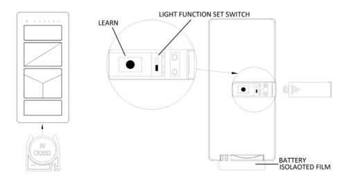
Step: 2. Hold the "LEARN" button for over 5 seconds, once the receiver has detected the frequency, the receiver will make sound, Bi Bi, twice. This will indicate the receiver has learned the frequency that was previously selected on the transmitter.
