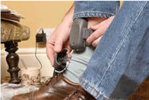
The BluTag® is easily installed by simply sizing the ankle and clicking in a premeasured tamper resistant fiber optic strap. If the fiber optic light is interrupted a tamper notice is sent to the officer.
