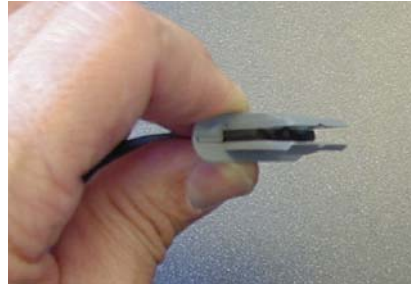
Incorrect alignment – end of strap and clips are not flush.
