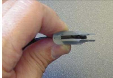
**Incorrect alignment** – end of strap and clips are not flush.
