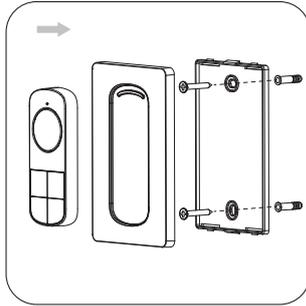
Screw on the faceplate bracket, then snap the faceplate cover onto the bracket. Then place the remote controller into the groove of the faceplate.
