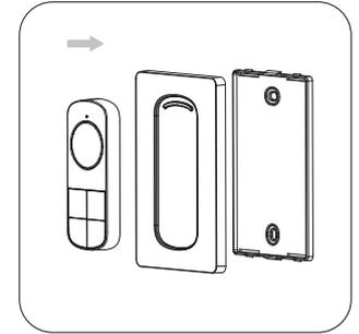
Snap the faceplate cover onto the bracket. Then place the remote controller into the groove of the faceplate.
