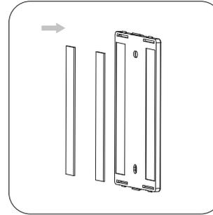
Apply adhesive tape to the groove of the faceplate bracket's back. Then mount the bracket to the wall.
