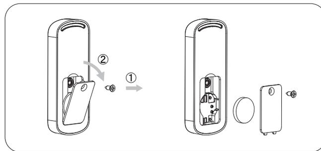
Remove the back cover of remote using the screwdriver to change the CR2032 battery.
