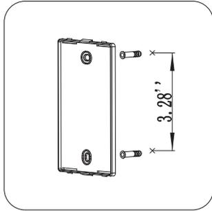
Mark the appropriate two keyhole locations. Drill two holes 3.28" apart using 15/64" size drill bit. Insert drywall anchors.
