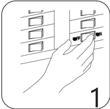
Turn off power source at the main circuit breaker or fuse box.
