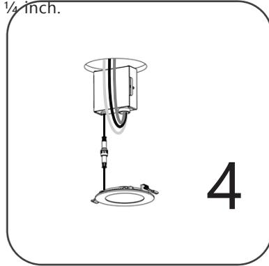
Place the junction box on the ceiling through cur hole. Connect the light with junction box with the connector.
