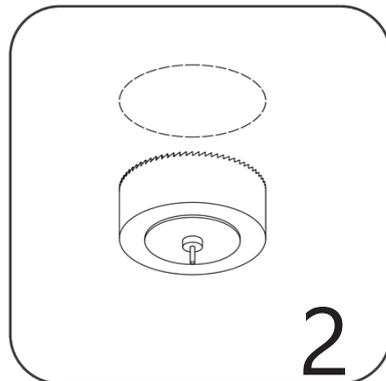
Drill hole in ceiling and prepare supply wire. Hole size CFIXCNLR4S1/ CFIXCNLR4C1 4 ¼ inch, CFIXCNLR6S1/ CFIXCNLR6C1 6 ¼ inch.
