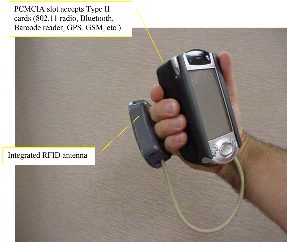
SMR-640P MobileReader connected to PDA handheld
