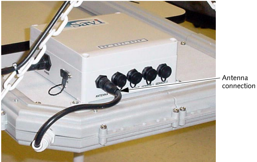
Figure 2-5 Model SP-600-201 Signpost Antenna Connection
