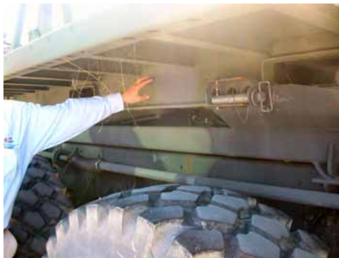
Figure 1 Alternative location for mounting SaviTag ST-614/ST-615 to CROP.
