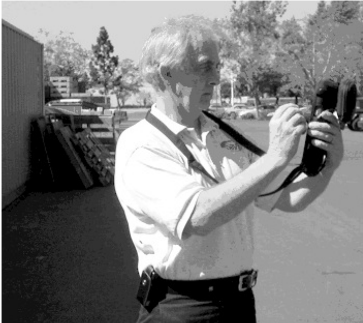
Figure 2-3 Hold the mobile reader at eye level and parallel to your body for optimal tag collection
