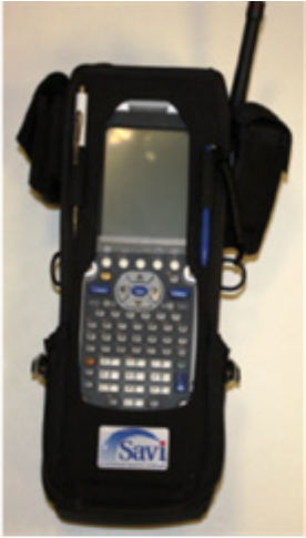
Intermec CK61G Mobile Computer enclosed in a soft case (with boot adapter and Savi Mobile Reader SMR-650 attached)
