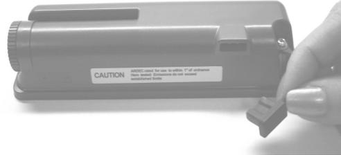
4. Insert Savi Tag Write Cable STA-1030 or Savi Tag Write Cable Adapter STA-1031, with the LED up, into the tag commissioning port. Start the tag commissioning application. The LED is lit when the application writes data to the tag.
