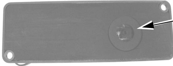
The temperature sensor inside the tag gauges the surrounding environment's temperature when air passes through this vent
