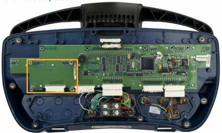
2/ Install TR02 intended for control pult. Tighten the supplied screws\*, normally 4
