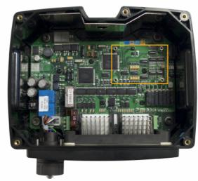
5/ Install TR02 intended for Receiver box and tighten supplied screws\*, normally 4.
