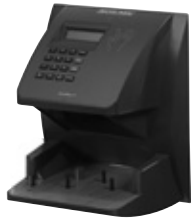
HandKey-2 Hand Geometry Reader
