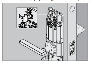
5. Remove the retention key. Remove the top bracket. Then, tilt the Module back and pull up to remove.
