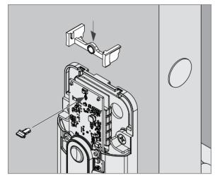
8. Reinstall the battery holder and retainer.
