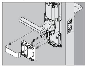
4. Release retention key by turning to the vertical position.
