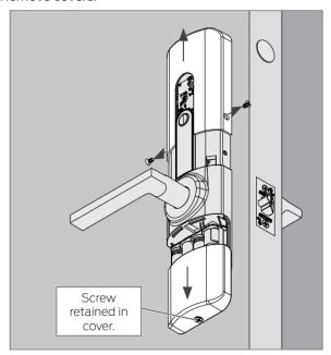
3. Remove battery retainer and holder.
