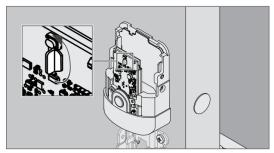
5. Remove the retention key. Then, tilt the Module back and lift up to remove.
