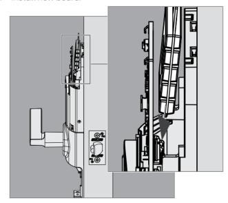
7. Reinstall the bracket and then the retention key.
