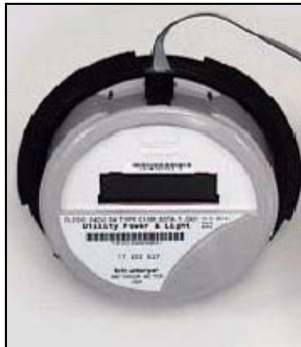
Figure 7.3 C1SC/CN1SC Programming Port Location
