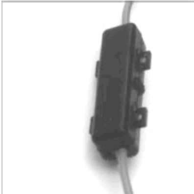
Figure 2.18 A Completed Splice
