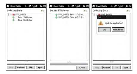
The next screen gives the information about the status of reading the devices. With the "Skip" button it is possible to skip the reading to the next logger. When done the information can be send to the ftp-server by pressing the "FTP" button. The data files (\*.dat files) can be imported by Diver-Offices. Quitting the application is done by the "Quit" button.
