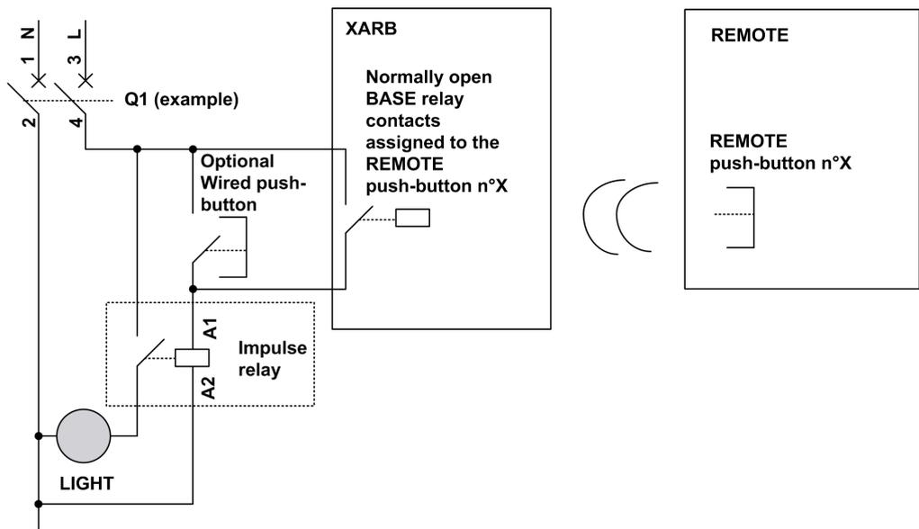
**NOTE:** Schneider Electric offers modular impulse relays which are bistable switches designed to control load power mainly for lighting applications.
