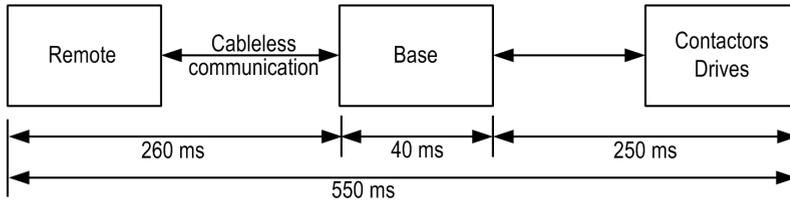
So 250 ms are allocated for contactors / drives of the hoisting system. The rest (300 ms) is allocated for Wireless Remote Control System. In consequences, the maximum response time of the Wireless Remote Control System is 300 ms for all safety functions in any configurations.
