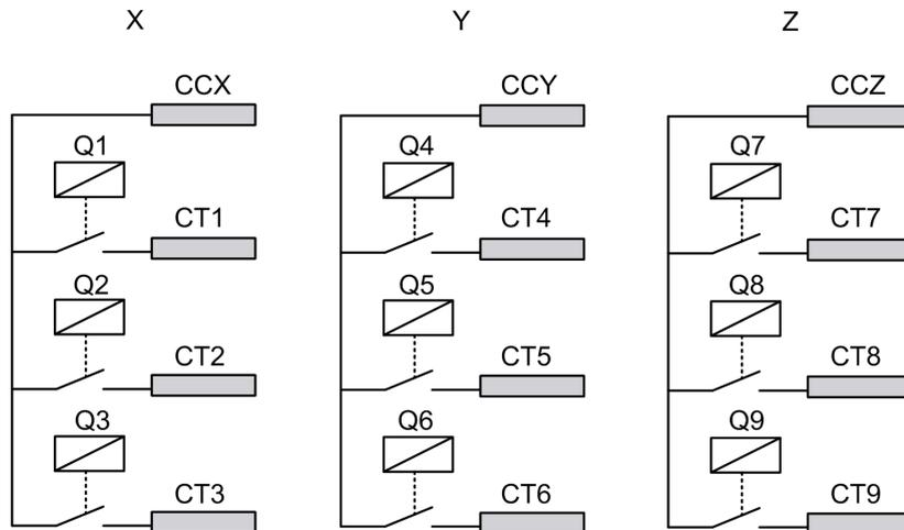
**Q10...Q16 motion/auxiliary relay wiring (NO type only)**
