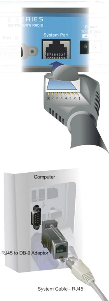
The TVIEW+ Cable is a standard CAT 5 RJ-45 (Male) to RJ-45 (Male) patch cable. It is intended for RS232 serial communications only and should not be connected directly into an ethernet port of a PC. The Cable must be used in conjunction with the RJ-45 to DB9 Adaptor.
