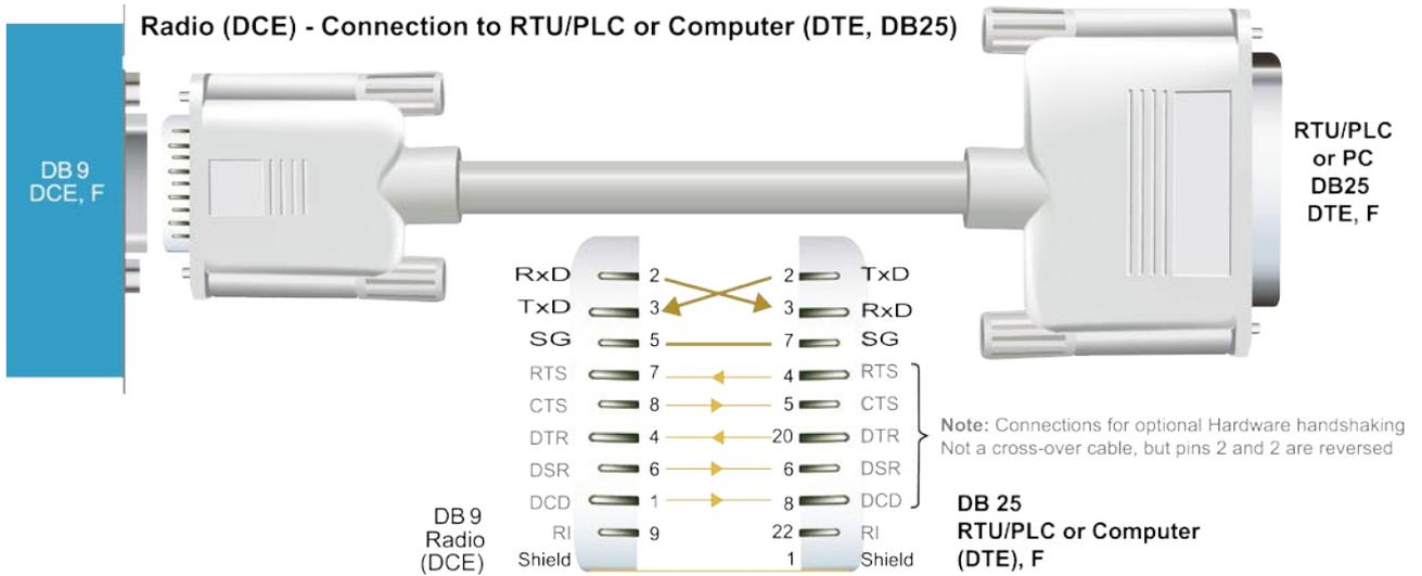
**RS232 Connector Pin outs (DCE)
