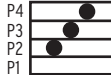
Figure 3.10 FCI Status Summary–No Tripped FCI(s) Indication in Summary, Row/Column, or Morse Code Mode
