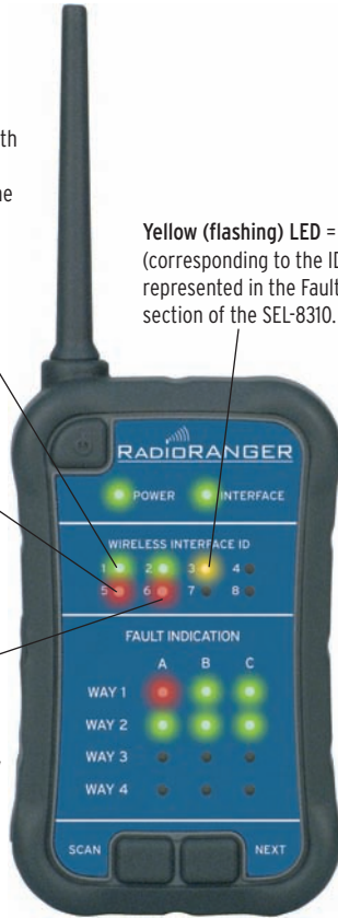
Figure 3.16 Wireless Interface ID LED Color Descriptions
