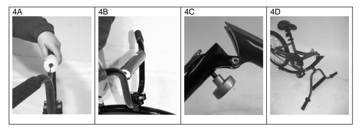
Check to see if the handlebar pad is properly attached. If it is not, follow steps 4A and 4B.
