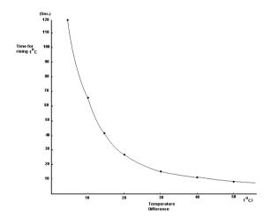
Temperature Rising (Descending) Speed vs. the Temperature Difference
