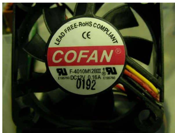
Figure 121: Dual Ball Bearing Fan
